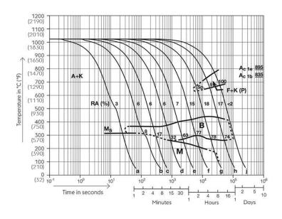
Austenitising temperature:  $1025^{\circ}C$  (1877°F) Holding time: 15 minutes 5...100 phase percentages 0.5...180 cooling parameter, i.e. duration of cooling from 800 - 500°C (1472-932°F) in s x 10<sup>-2</sup>
