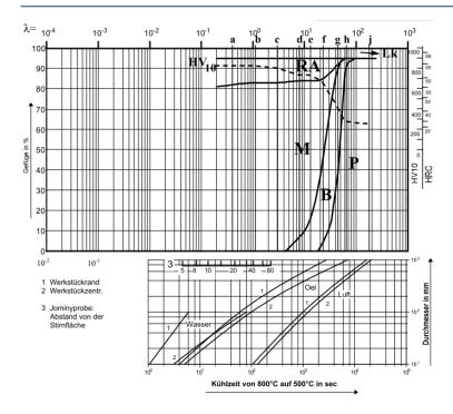
HV10... Vickers Hardness Lk... Ledeburite carbide RA... Residual austenite
