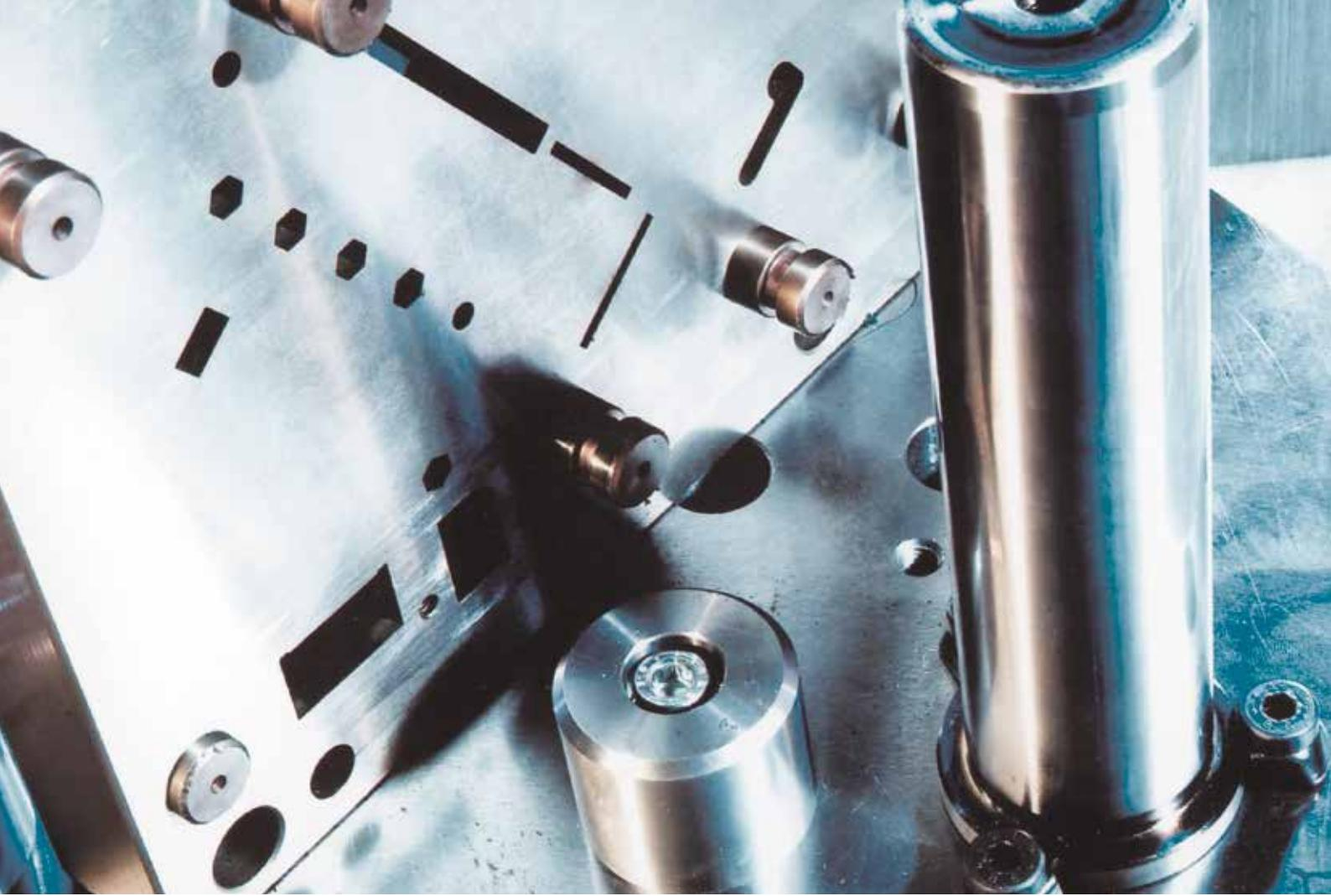
Alloying with aluminum improves the tribo-system so that surface oxide passivation occurs. This passivation layer reduces the tool's adhesion tendencies in use.
