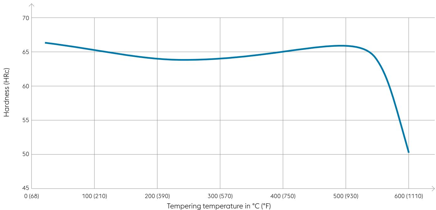
Vacuum hardening: 1050°C (1920°F) / 30 min / N<sub>2</sub>, 5 bar
