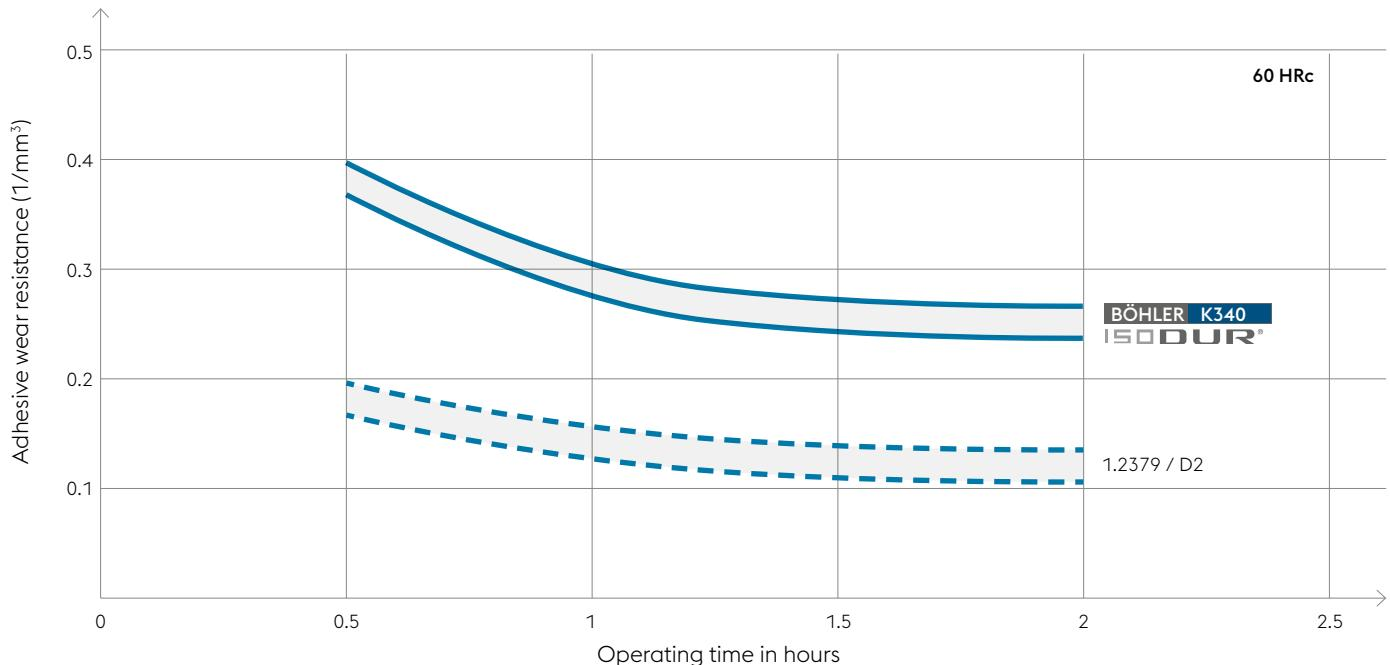
determined by the pin-on-disc test
