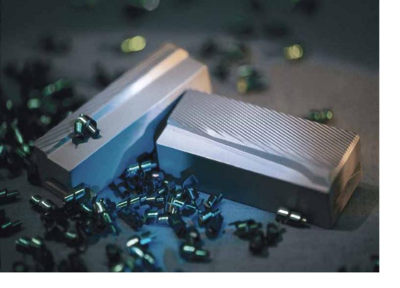
Alloying with aluminum improves the tribo-system so that surface oxide passivation occurs. This passivation layer reduces the tool's adhesion tendencies in use.
