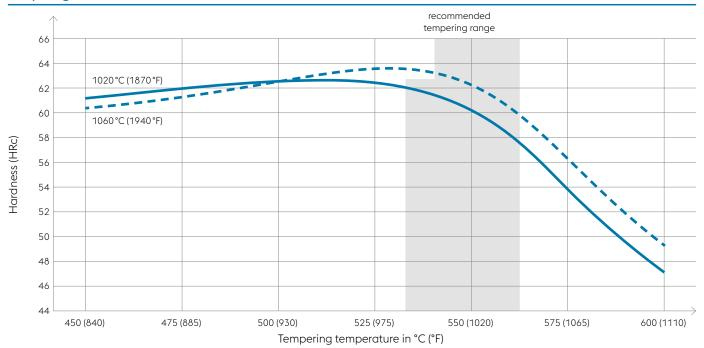
Specimen size: square 20 mm (0.79 inch) Hardened in vacuum,  $\mathrm{N}_{\mathrm{2}}$  cooling 5 bar
